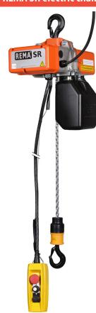
Series SR 230 V electric chain hoists are available in several designs and they have the same advantages as standard 400V models i.e. safety slip clutch/brake assembly, low construc-tional height etc. For the 1-phase connection, wire having a minimum cross-section of 2.5 mm<sup>2</sup>. For power distribution at building sites, use connection cables of as short as possible to minimize voltage drop.
